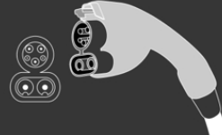
SAE J1772 DC CCS Combo 1 Connector Type 1
